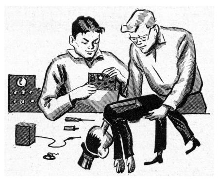
can spring-load his jaw so that it's normally closed and a pull on this cord will open it. Audio voltage picked off the receiver and rectified with a germanium rectifier will produce pulses of d.c., which can drive a high-current transistor with a solenoid in its output circuit. This solenoid will give a yank on the jaw cord with every syllable of the voice picked up by the receiver."
